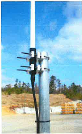
Figure 84 – RF Antenna to Mast
